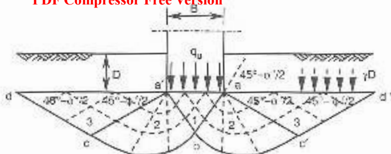
Figure 10.1. Failure mechanism for frictionless strip footing.
